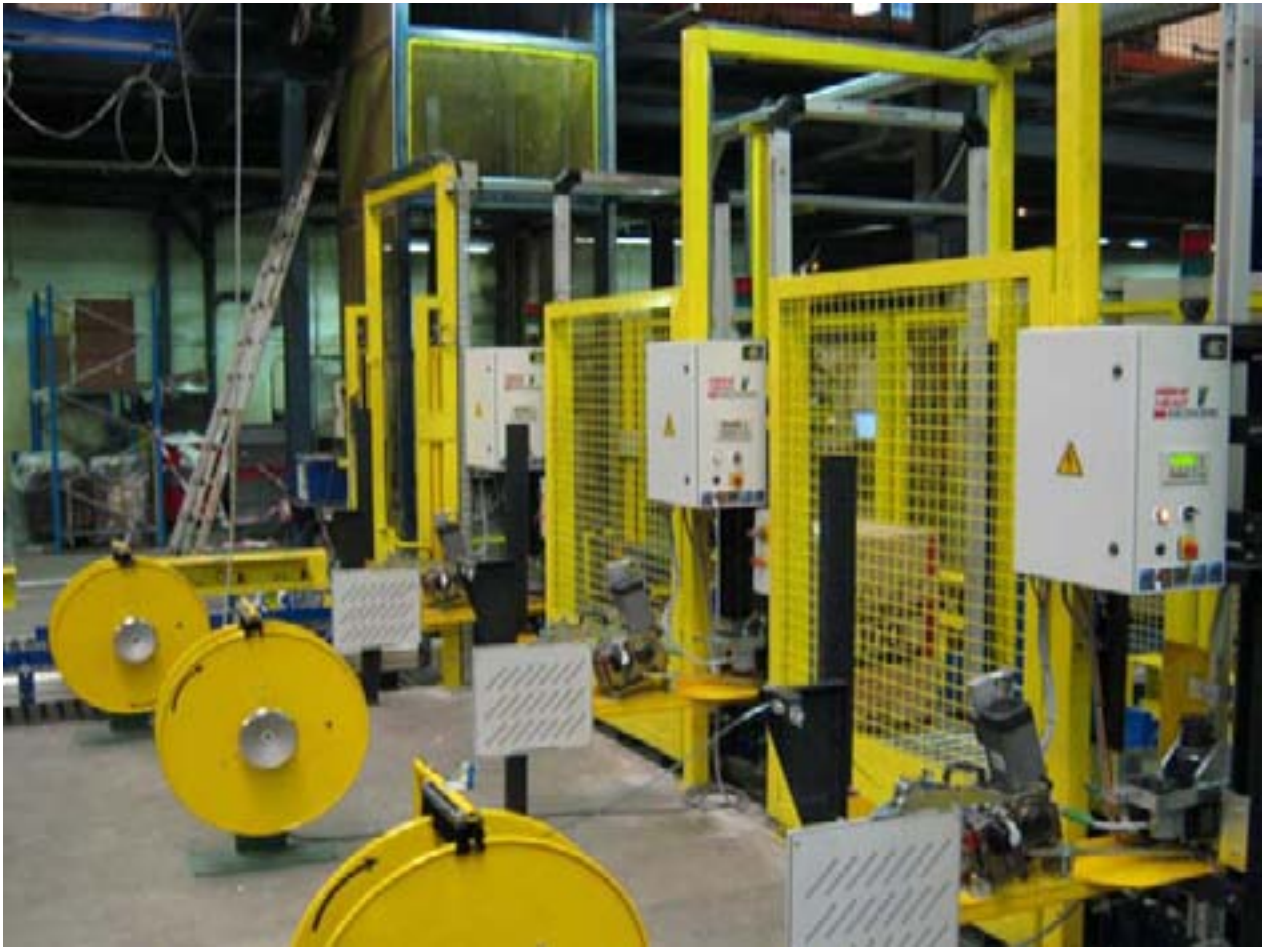
MH-V Side-Seal Machine shown in a high through-put production plant strapping packaged domestic appliances
