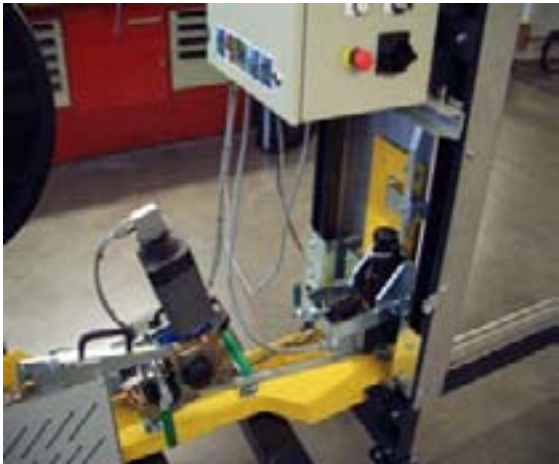
Easy access MH feed and take up and MH Strap sealer module on MH-V model
