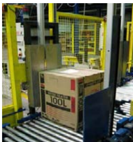
Small appliance pack being strapped in large chute machine, it can accommodate varying load heights
